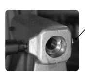
**Note**. Do **not** adjust the screws at the side of the tailstock as these are factory set.
