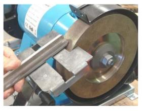
Roughing Gouge & Round End Scraper -  $66^{\circ}$
