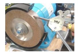
Flat profile spindle gouges - 33°
